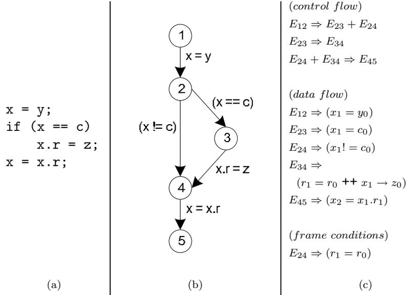
Figure 17. Translating sample code to Alloy: (a) a piece of code, (b) corresponding CFG, (c) Alloy encoding
